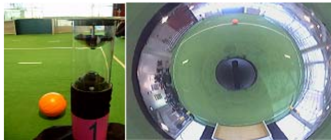
Figure 4 : Omni directional vision system installed on each robot
