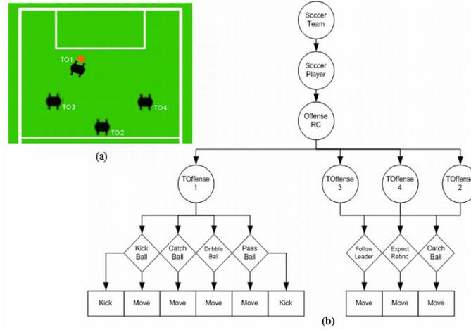
Figure 5. Dynamic offensive formation (a) and corresponding decision machine (b).
