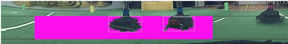
**Fig. 6 :** Example of results obtained with obstacle detection mechanism. Obstacles are bounded with white rectangles and safe regions are marked with magenta color.
