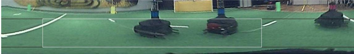
**Fig. 5 :** Obstacle detection area is mapped to a rectangle on the panoramic image.
